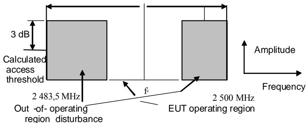
**Figure 1: Spectrum Mask for Test of clauses 5.3.3.2.1, 5.3.3.2.2 and 5.3.3.2.3**
