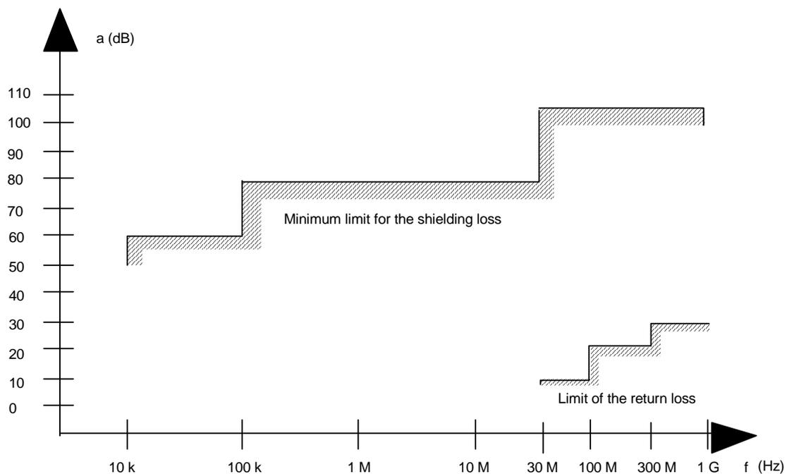
Figure B.5: Specification for shielding and reflections
