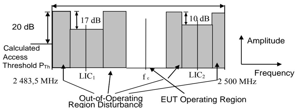
Figure 4: Spectrum Mask for Test
