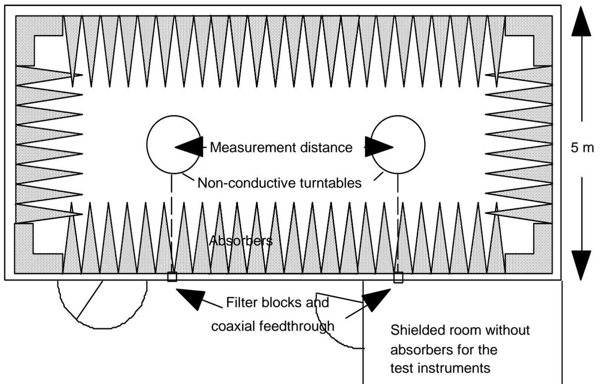
Figure B.6: Example of construction of an anechoic shielded chamber
